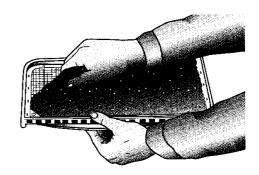
NOTE: Do not operate the dryer without the lint filter in place.
